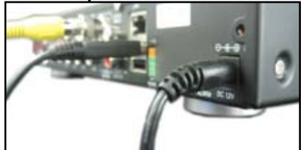
Connect to a power source to turn on DVR
